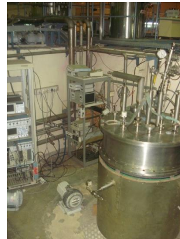
High Pressure Rinsing (HPR) facility installed in a Class-100 Clean Room; photograph shows HPR of a QWR in progress.
