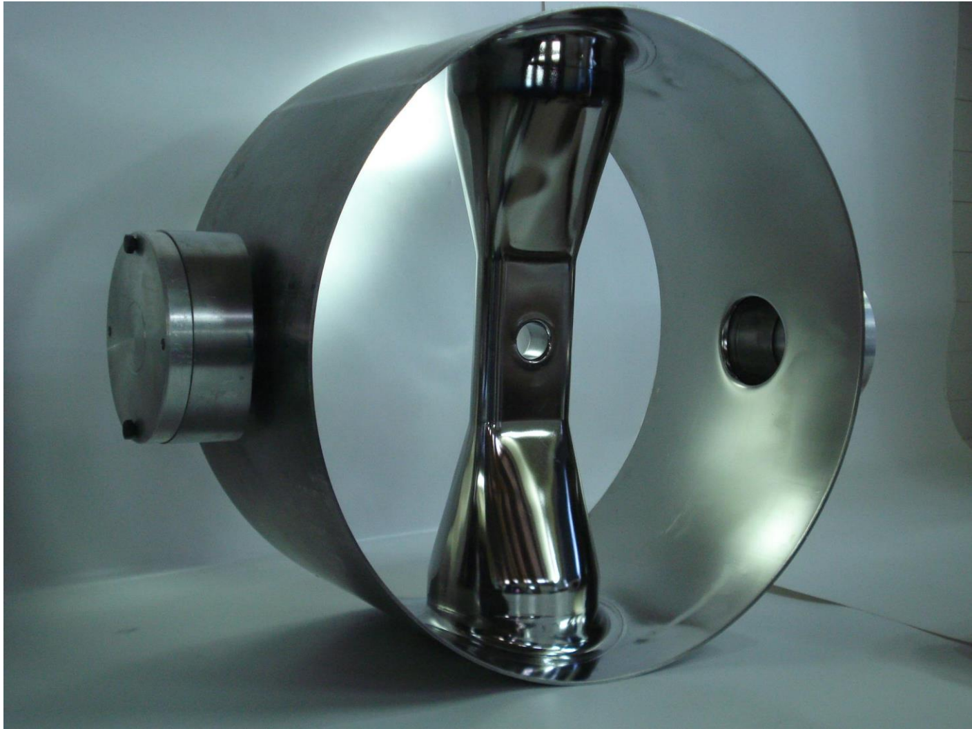
Completed Spoke and Shell assembly.
