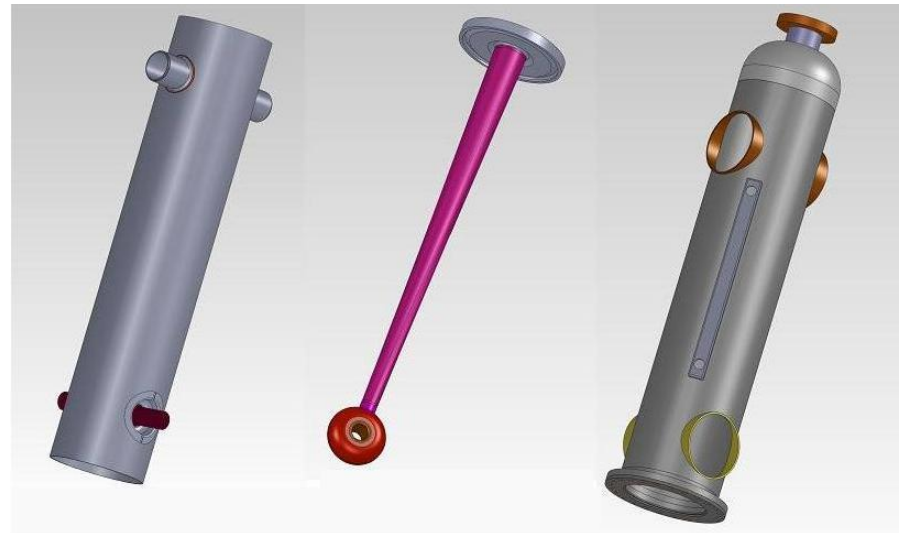
Major sub-assemblies of the Low Beta Resonator: niobium outer housing, tapered niobium central conductor and top flange, and stainless steel outer helium vessel.
