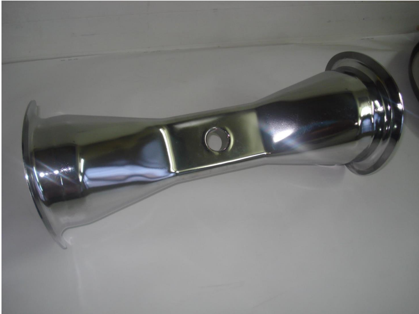
Niobium Spoke assembly after electropolishing.
