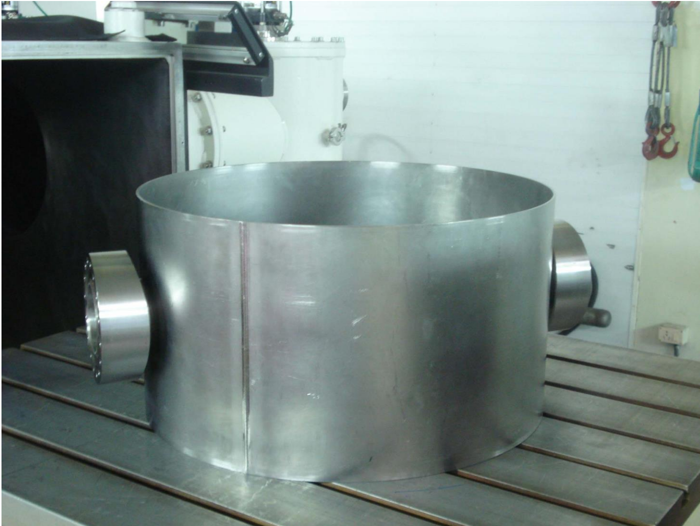
SSR1 niobium Outer Shell along with its Coupler Ports.
