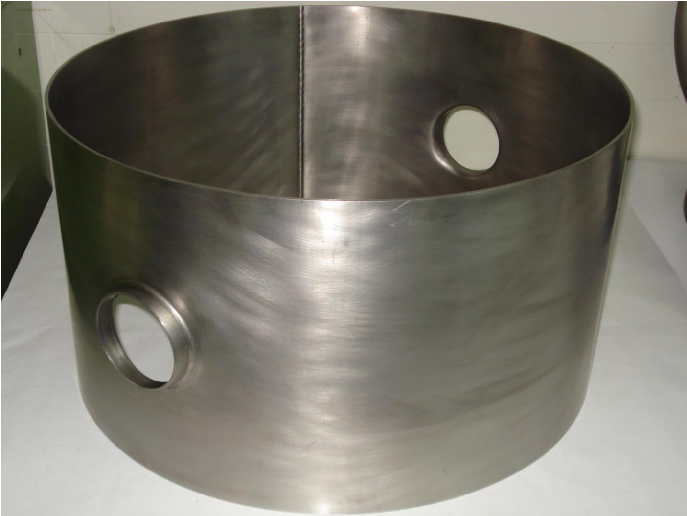
An Outer Shell after pulling out both the Coupler Ports.
