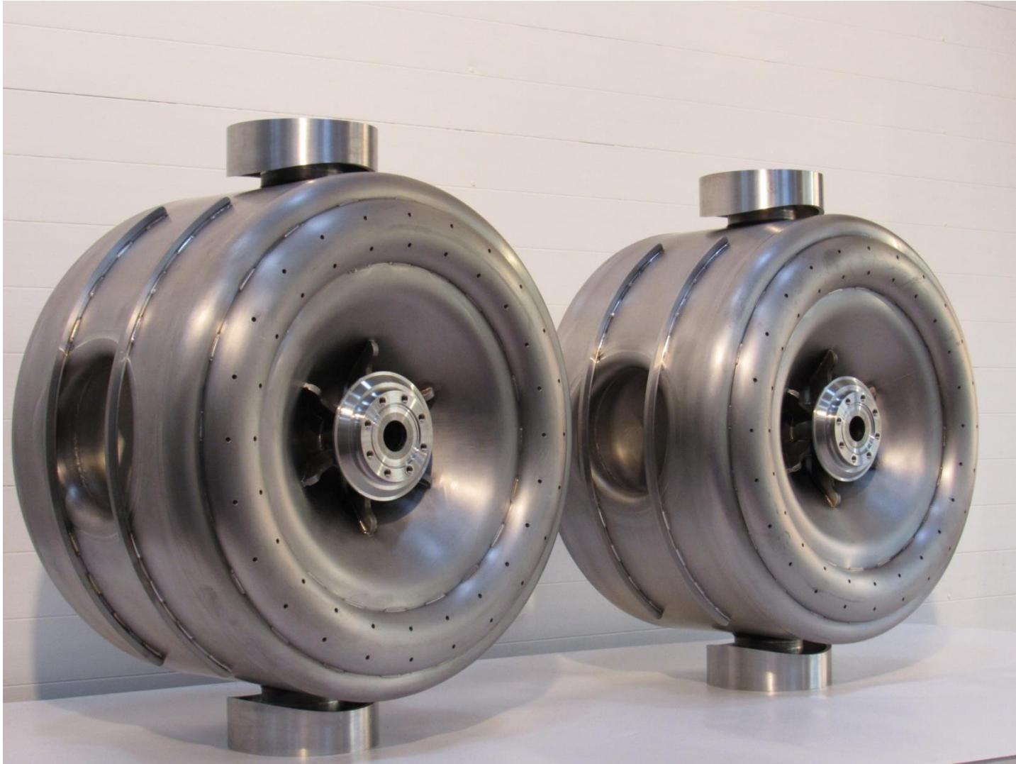
The two SSR1 Niobium Spoke Resonators developed at IUAC.
