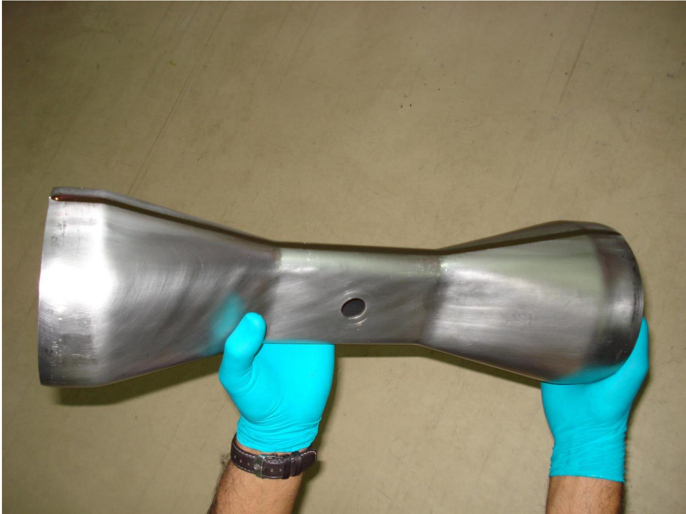
Niobium Spoke assembly after EBW of the two halves.
