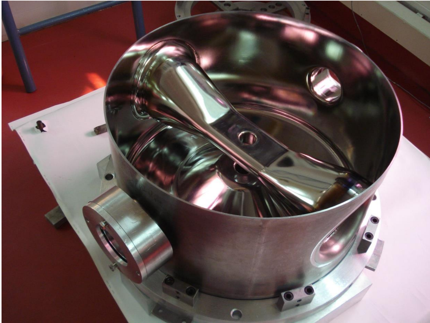
A Niobium SSR1 resonator just before completion.
