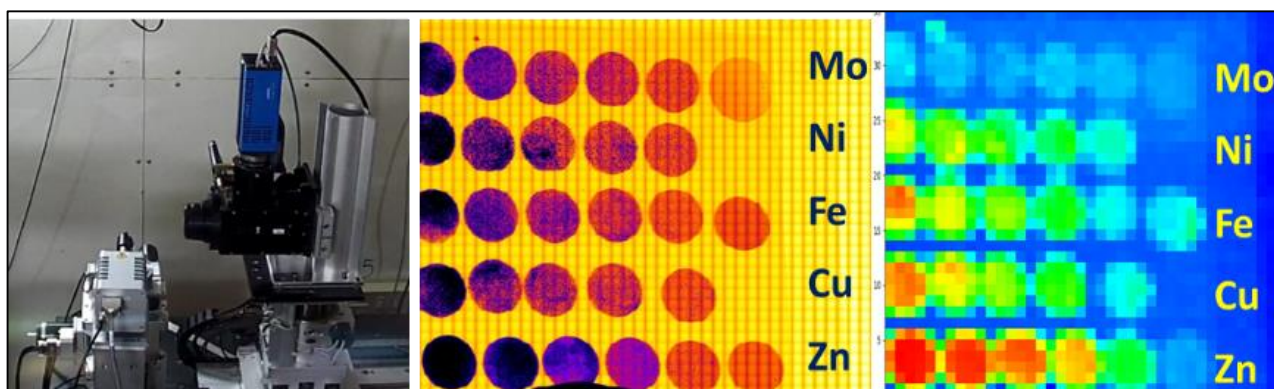
Combined transmission & elemental mapping experimental set-up at BL-04 with transmission image and fluorescence based elemental concentration
