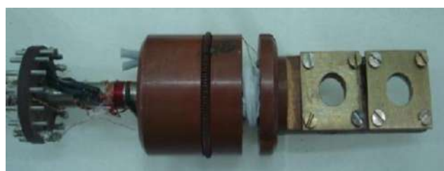
Fig. T.1.12: Photograph of the sample holder attached to the insert used for loading samples inside the cryostat shown in Fig. T.1.11.
