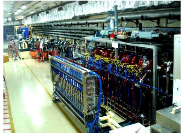
Fig. T.1.3: Photograph of the IR-FEL at RRCAT which lases at 12-50 \mu m.
