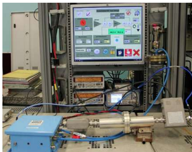
Fig. P.6.2: Automated RF Test bench for testing absorber sample at high power
