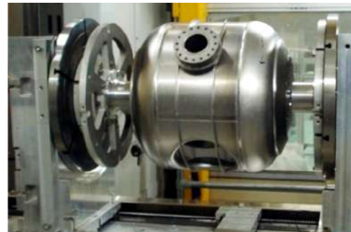
Fig. P.3.3: SSR-2 Cavity assembly after final EB welding
