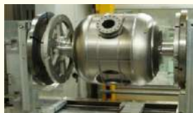
Indigenously developed SSR-2 SCRF Cavity for PIP-II project
