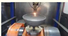
LAM-DED based manufacturing of thin wall dome structure
