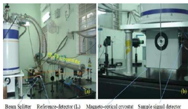
Fig. T.1.11: Experimental set up used to measure the IR-FEL light absorption as a function of temperature and magnetic field.
