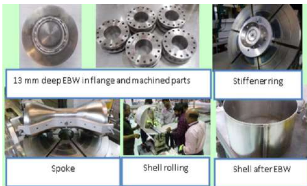
Fig.P.3.2: Various components of SSR-2 cavity
