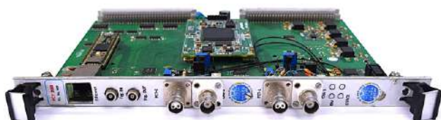
Fig. E.6.1: In-house developed VME32 FCT card
