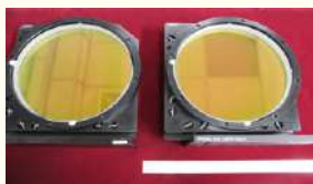
High transmission, high LIDT AR coated optics of 200 mm diameter
