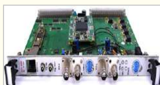
Indigenously developed VME32 DAQ card for FCT interface
