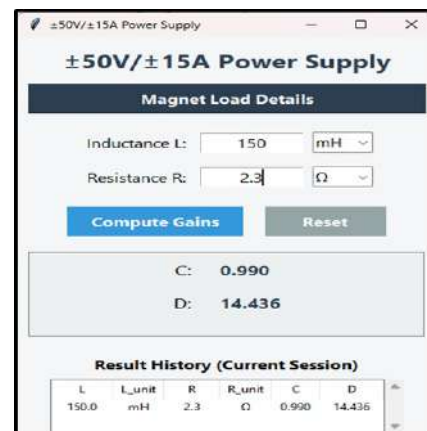
Fig. E.5.3: GUI of software for controller gains
