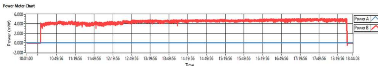
Fig. T.1.5: Stability of the radiation emitted from IR-FEL, as measured at the user laboratory.
