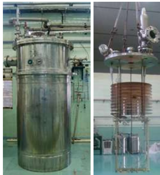
Fig. P.4.2: (a) Test Cryostat, (b) Insert assembly.
