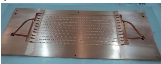
Fig. I.2.1: Machined wavy grooves on the grid plate
