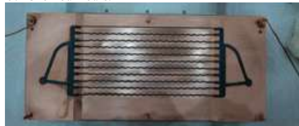
Fig. I.2.2: Wax filled wavy grooves on the grid plate
