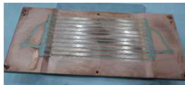
Fig. I.2.3: Wax filled wavy grooves coated with silver
