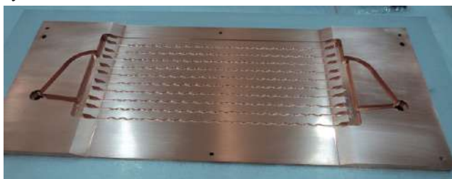
Fig. I.2.1: Machined wavy grooves on the grid plate
