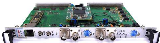
Fig. E.6.1: In-house developed VME32 FCT card
