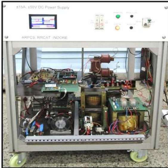
Fig. E.5.1: FPGA controlled bipolar power supply with HMI
