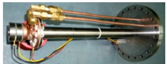
Fig. T.1.16: In-house designed and developed water-cooled, high vacuum compatible Faraday cup for beam current measurement.
