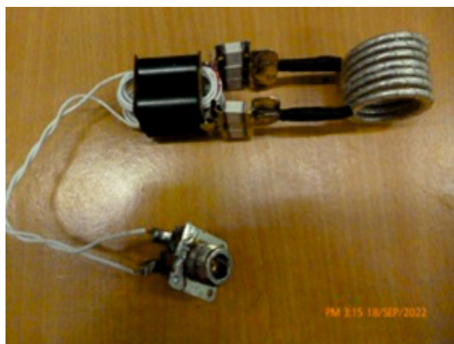
Fig. T.1.10: 13.56 MHz RF ignition antenna and transformer based matching network.
