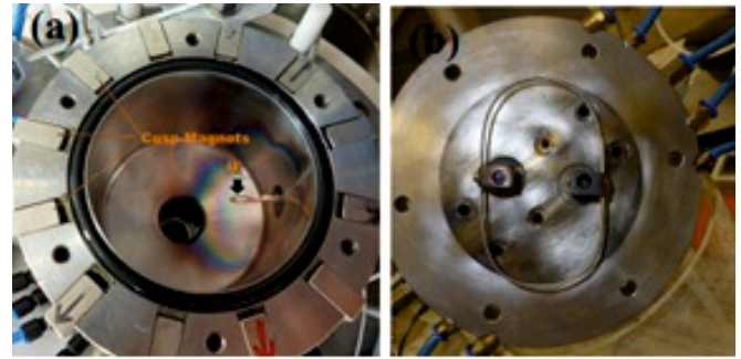
Fig. T.1.4: (a) Multi-cusp plasma chamber and (b) back flange with oval shaped tungsten filament.
