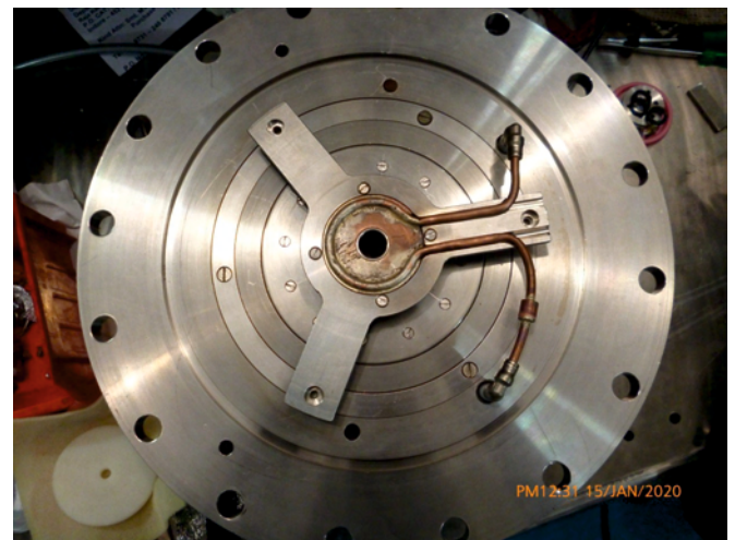
Fig. T.1.15: Assembly of water-cooled high voltage and high vacuum compatible extraction electrode rated for 15 kVDC.
