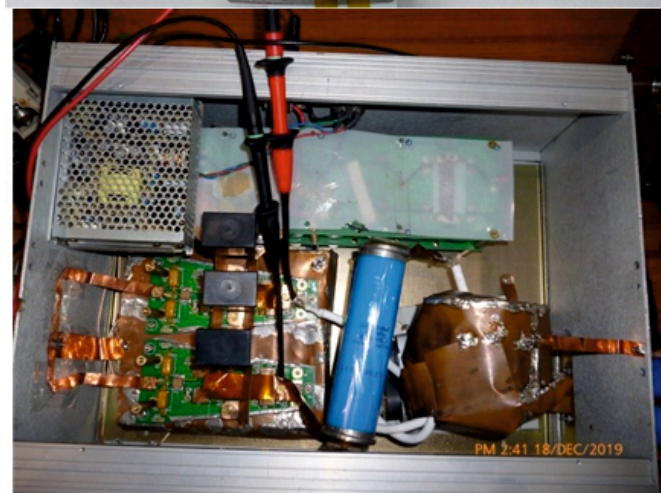
Fig. T.1.17: Developed 2 MHz RF source components and their assembly.
