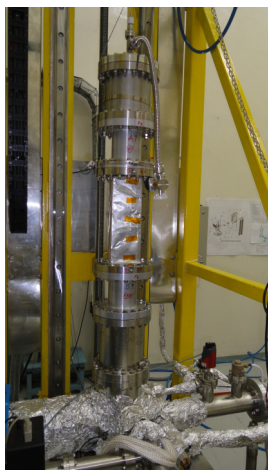
Fig. T.1.13: Coating facility integrated with alumina chamber for coating.
