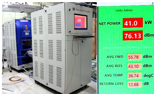
Photographs of the 40 kW, 650 MHz solid state RF amplifier (left) and snapshot of the measured RF power during rugged testing at RRCAT with 50 Ohms RF load (right).
