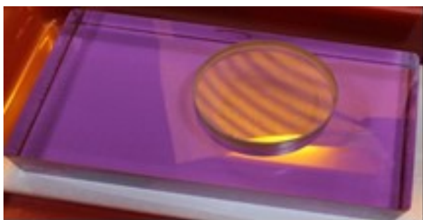
Fig. T.2.2: Photograph of polished Nd:glass slab.
