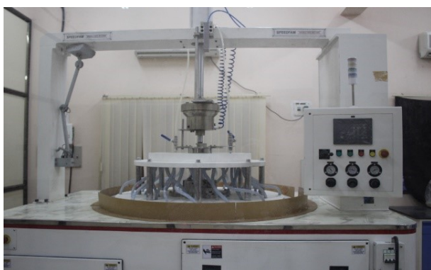
Fig. T.2.3: Double side optical polishing machine.
