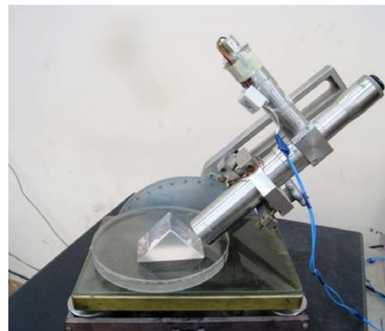
Fig. T.2.11: In-house developed autocollimator.
