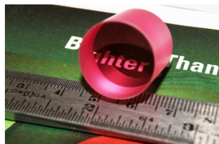
Fig. T.2.4: Polished Ti:sapphire crystal of size dia. 20 mm x 15 mm length.
