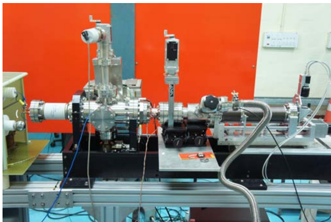
Fig. A.4.1: Characterisation of low emittance gun on test stand.
