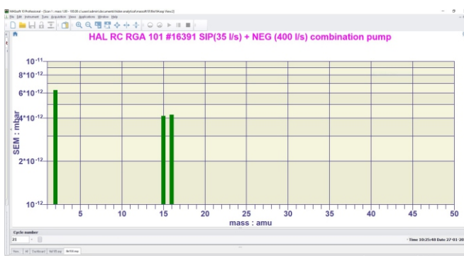
Fig. A.9.3: Residual gas spectrum scan at ultimate vacuum condition.
