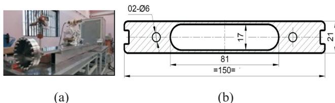
Fig. A.7.2: (a) Photograph, and, (b) cross section of vacuum chamber.
