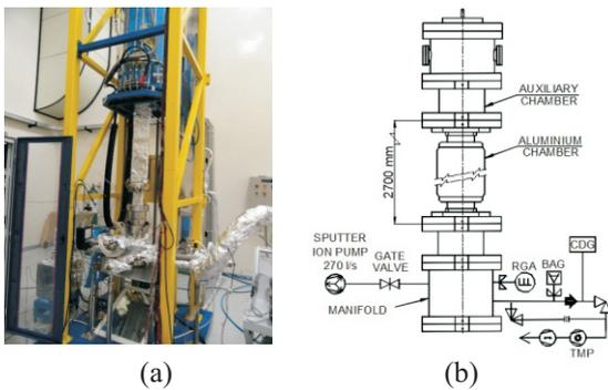
Fig. A.7.1: (a) Coating setup with vacuum chamber, and, (b) schematic of ultimate vacuum test setup.
