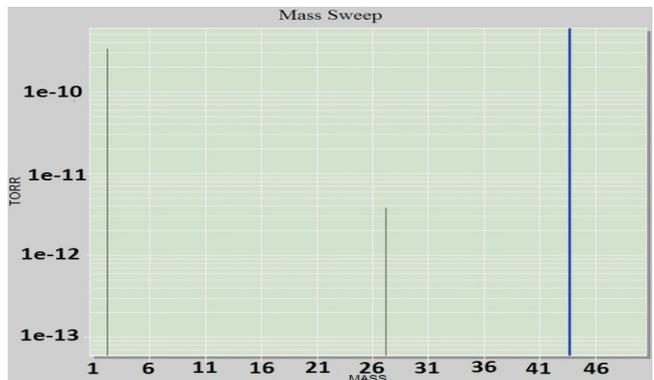
Fig. A.7.3: RGA spectrum of NEG activated chamber.
