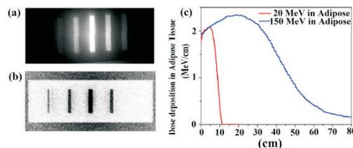
Fig. L.2.3: (a) Radiograph of a brass groove using 150 MeV energy. (b) Geant4 simulated radiographic image of brass groove. (c) Energy dose deposition rate in adipose tissue using Geant4 simulation for 20 MeV and 150 MeV energy electron beams.
