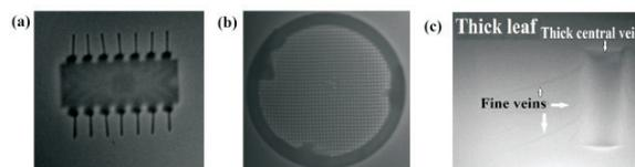
Fig. L.2.2: Radiographic images of (a) IC chip, (b) Cu mesh and (c) Thick leaf.
