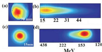
Fig. L.2.1: Electron beam profile and spectrum for Ar gas jet (a) and (b), and He gas jet (c) and (d), respectively.
