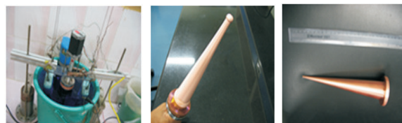
Fig. A.7.3: (a) Electroforming set up. (b) Electroformed copper. (c) Machined free standing copper cone.
