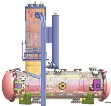
Fig. A.6.1: 3D model of HTS cryostat designed at RRCAT.
