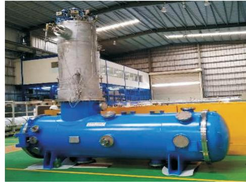
Fig. A.6.2: Fabricated HTS cryostat with feedcan.
