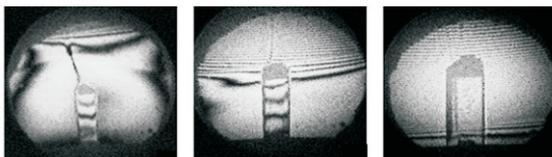
Fig. T.2.8: Progressive stages of concentration gradient during free convection growth of KDP crystal.
