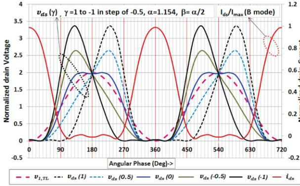
Fig. T.3.6: Drain voltage and current waveforms for Continuous Class F operation.
