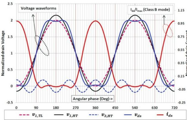
Fig. T.3.4: Drain voltage and current waveforms for third harmonic waveform shaping.
