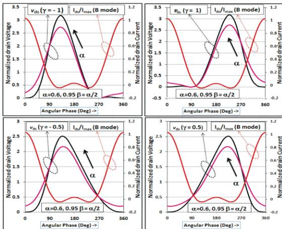
Fig. T.3.7: Different drain voltage waveform for Extended Continuous Class F mode.
