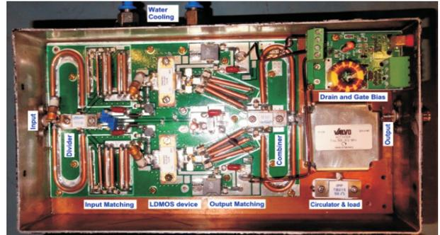
Fig. T.3.10: Fabricated 500 W PA module.
