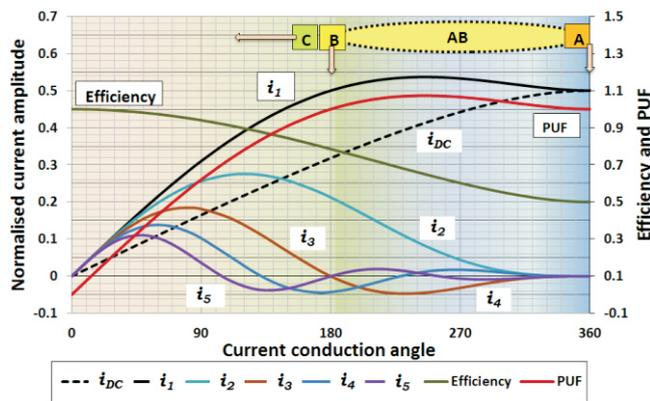
Fig. T.3.2: Normalized current components for tuned load PA operation.
