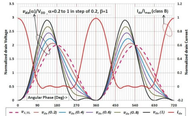
Fig. T.3.8: Drain voltage waveform for different values of  $\alpha$  and constant value of  $\beta$ .
