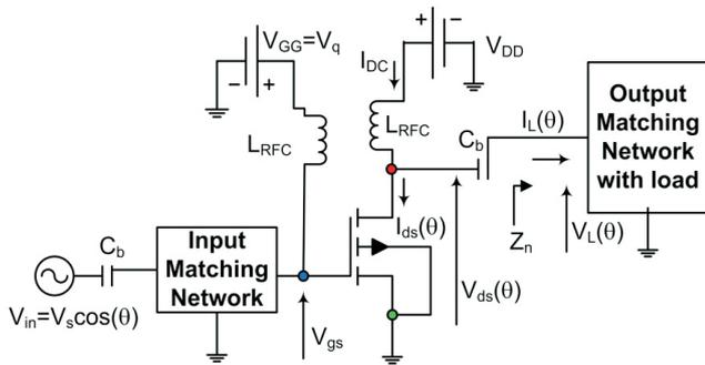
Fig. T.3.1: PA scheme with bias and impedance matching networks.
