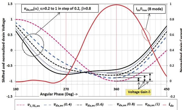
Fig. T.3.9: Shifted and normalized drain voltage waveform for different values of  $\alpha$  in CJ mode.
