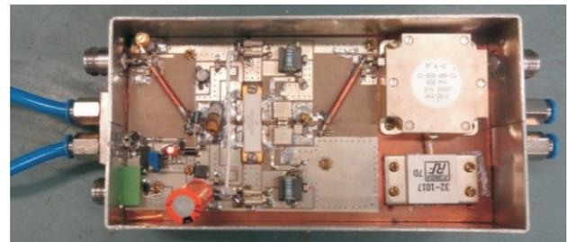
Fig. T.3.13: Fabricated PA in Extended Continuous Class F mode.
