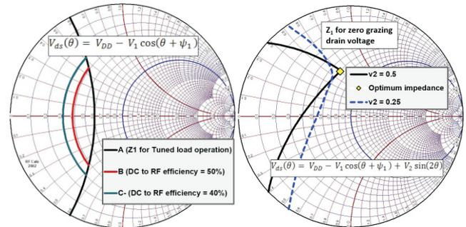
Fig. T.3.3: Design curves plotted on Smith charts for non-zero crossing drain voltage waveforms.
