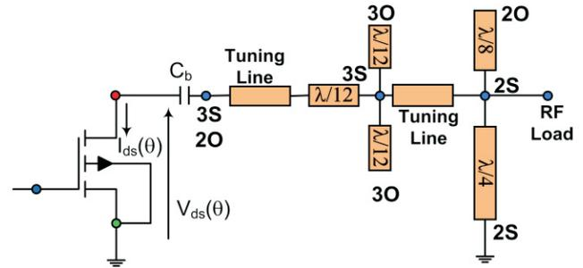
Fig. T.3.5: Possible output matching network for third harmonic tuned case.
