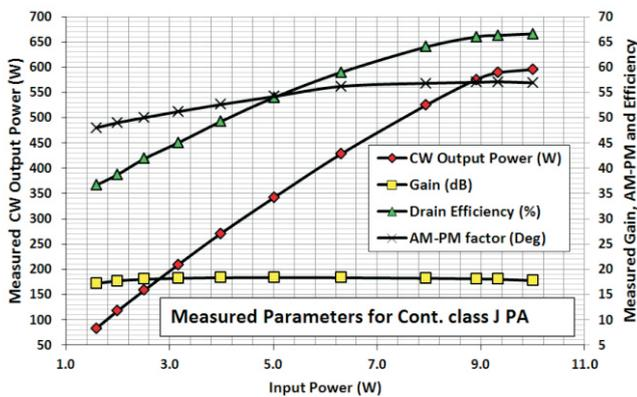
Fig. T.3.11: Measured RF performance of 500 W PA module at 505.8 MHz.
