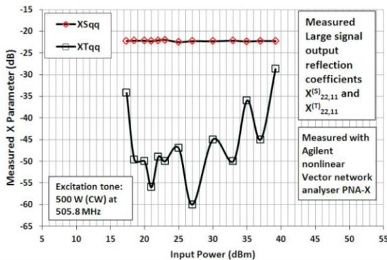
Fig. T.3.12: Measured X parameter for at 500 W.
