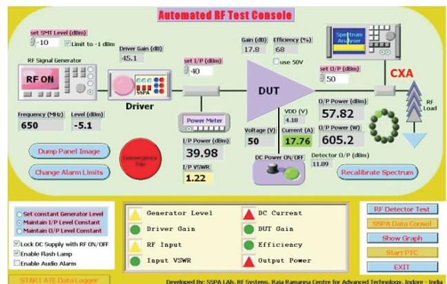
Fig. T.3.14: Measured high power parameters of 650 MHz PA.
