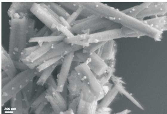
Fig. L.8.1: SEM image of ZnO nanorods decorated with Au nanoparticles.
