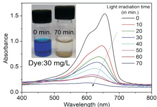
Fig. L.8.2: Variation of methylene blue dye absorbance for different light irradiation time (Inset: Colour of the dye solution, before and after light irradiation).
