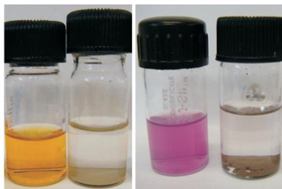
Fig. L.8.3: Photographs of (left) methyl orange dye and (right) textile industry dye effluent, before and after light irradiation in presence of nanocomposites.
