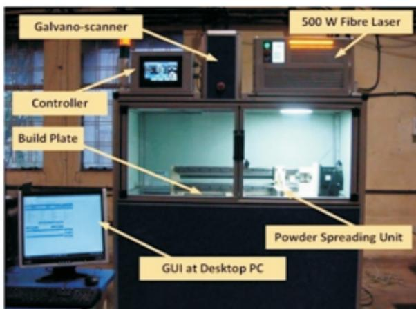
Fig. L.3.1: 500 W fibre laser based LAM-PBF system.
