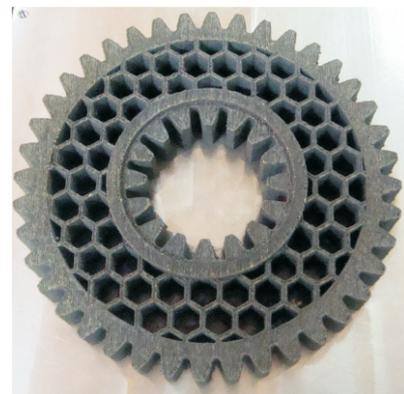
Fig. L.3.3: External and internal geared geometry with honeycomb core.
