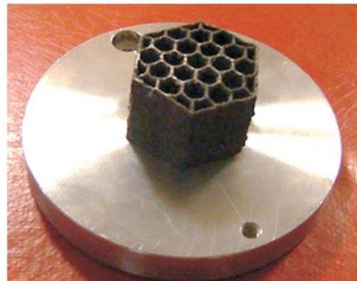
Fig. L.3.2: Hexagon channeled nipple.
