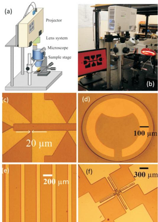
*Fig. L.1.1: (a) Schematic and (b) photograph of experimental arrangement for maskless photolithography system. Photograph of (c) Hall bar of 2DEG sample, (d) detector structure, (e) laser diode arrays and (f) inverse spin Hall effect sample are shown, which are fabricated by the above system.*
