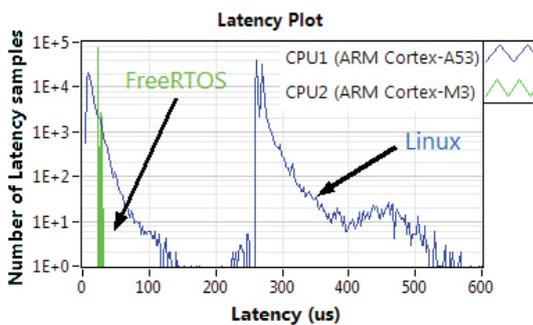
Fig. A.8.2: Measured interrupt latency for LINUX (CPU1) and RTOS (CPU2) on new VME CPU board.
