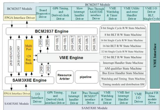
Fig. A.8.3: New VME CPU board software module block diagram and their interconnections.
