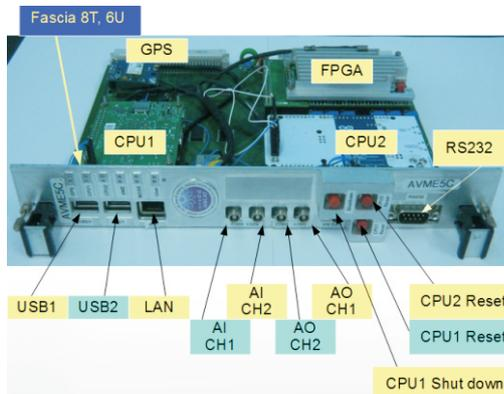
Fig. A.8.1: New VME CPU board interface details.
