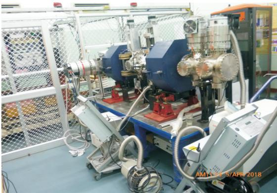
Fig. A.6.1: Experimental setup of H<sup>-</sup> ion source coupled with LEBT and beam diagnostics.
