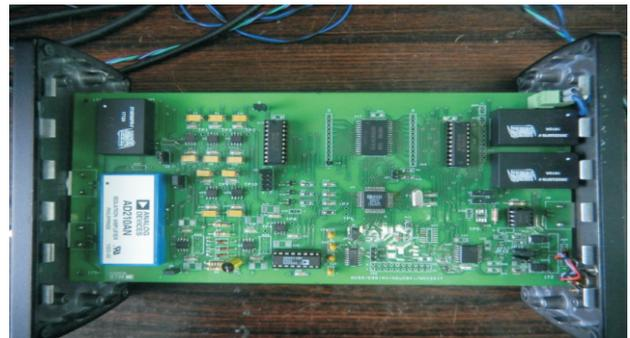
Fig. A.5.2: Photograph of the data acquisition system.
