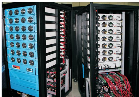
Fig. A.3.2: Photograph of 50 V, 700 A DC power supply.
