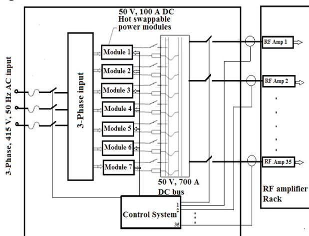
Fig. A.3.1: Scheme of 50 V, 700 A DC power supply.
