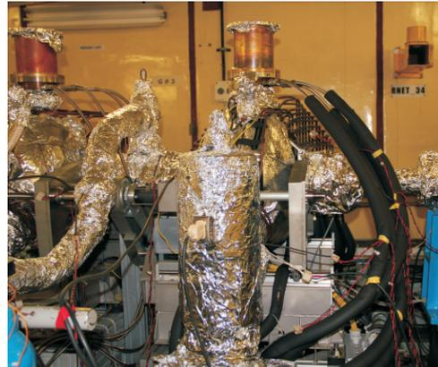
Fig. A.1.2: The sixth RF cavity along with vacuum system during baking.
