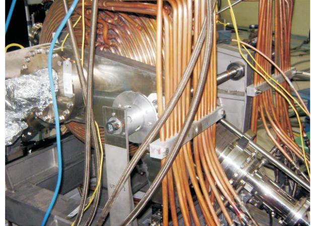
Fig. T.1.8: Cavity integrated with tuner and HOMFS
