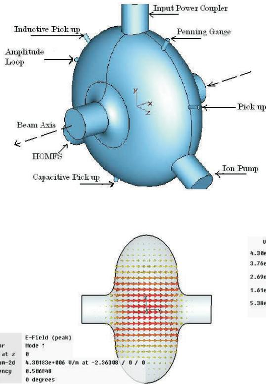
Fig. T.1.2: (a) View of the simulated cavity. (b) Electric field plot in RF cavity
