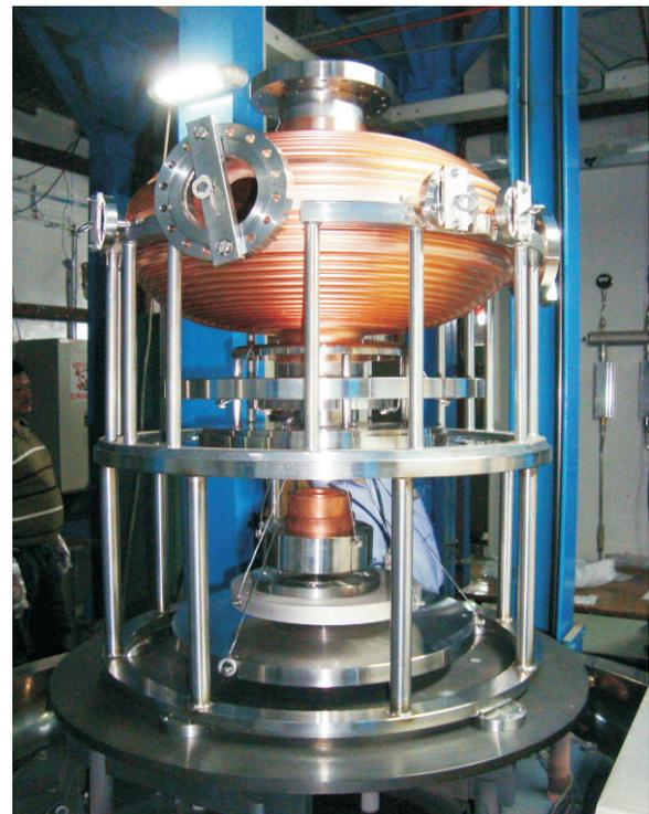
Fig. T.1.6: Pre-brazing assembly of ports with the cavity shell and its loading in the brazing fixture
