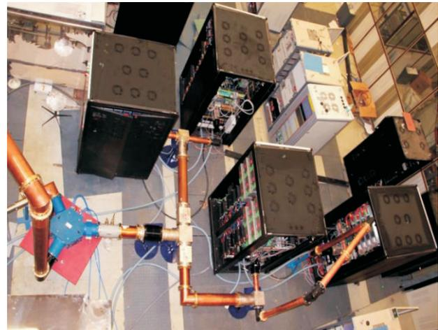
Fig. T.1.15: View of SSPA with transmission line system
