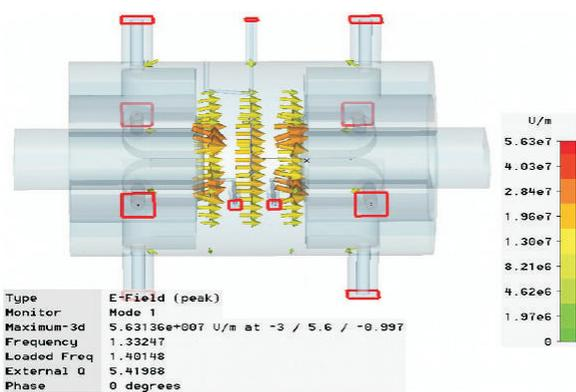
Fig. T.1.17: Simulated electric field for fundamental mode
