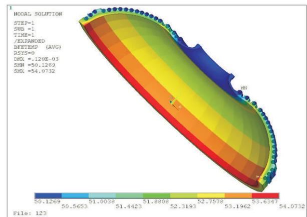
Fig. T.1.4: Temperature profile on the cavity wall
