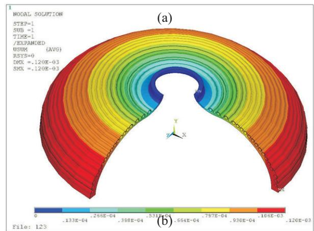
Fig. T.1.3: Deformation due to heat load
