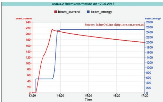
Fig. T.1.16: Indus-2 operation at 200 mA and 2.5 GeV
