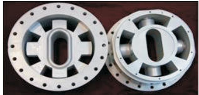
Fig. T.1.18: Machined parts of Kicker RF cavity
