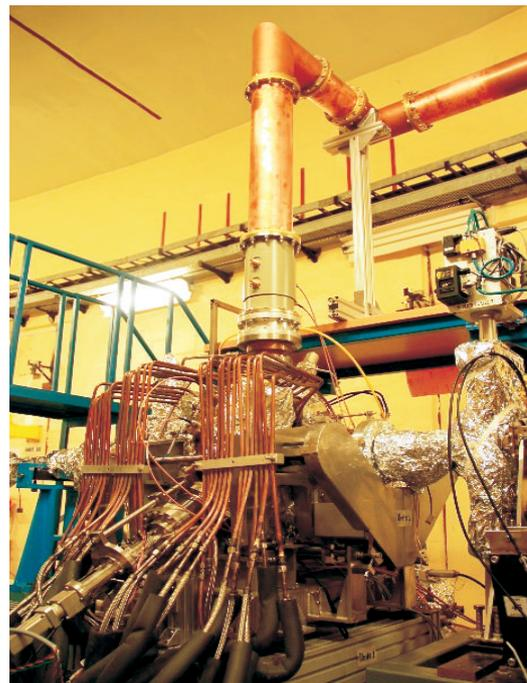
Fig. T.1.1: Indigenous RF cavity installed in Indus-2
