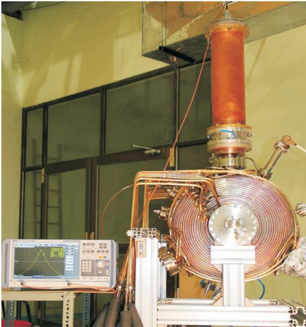
Fig. T.1.9: Coupling coefficient adjustment of RF cavity
