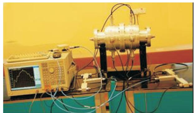
Fig. T.1.19: RF measurement set up with assembled cavity
