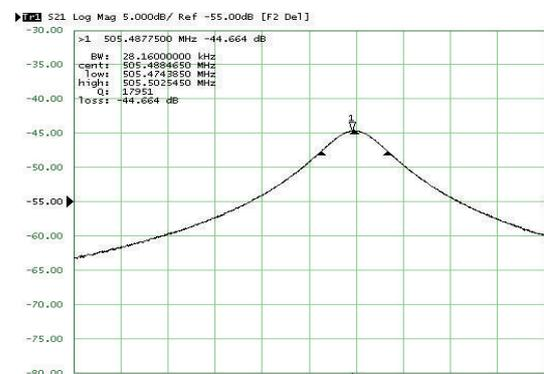
Fig. T.1.11: Snapshot of low power RF measurement
