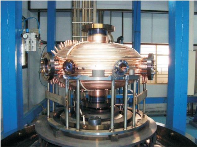
Fig. T.1.7: Cavity as brazed in the final stage on the furnace hearth with all cooling tubes
