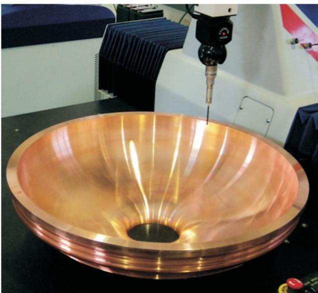
Fig. T.1.5: Inspection of half-cell on CMM
