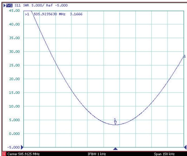
Fig. T.1.14: Snapshot of input power coupler coupling coefficient measurement
