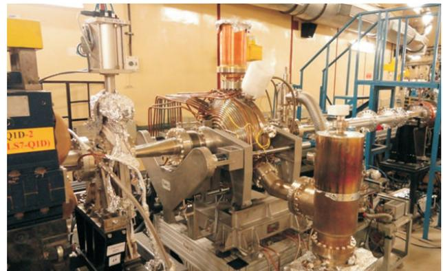
Fig. T.1.13: Upgraded LS-7 with indigenous RF cavity and vacuum system
