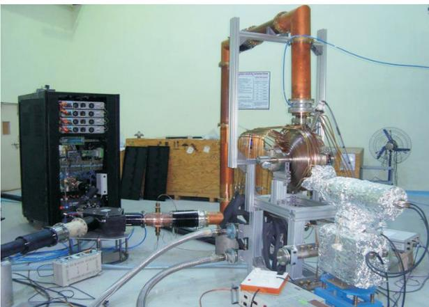
Fig. T.1.10: Set-up for RF conditioning and high power RF testing of the cavity
