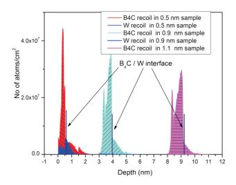
Fig.T.3.5: Recoil distribution of  $B_4C$  and W atoms when samples having top layer  $B_4C$  of 0.5, 0.9 and 1.1 nm thickness above 1.0 nm W layer is bombarded with 100 eV ions/neutrals. The recoil distribution graph has been shifted on X-axis (depth direction) for clarity.
