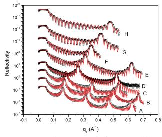
Fig. T.3.4: X-ray reflectivity curves both experimental (open circles) and fitted (solid lines) as a function of wave vector transfer  $'q_z(Å^{-1})$  for all the as deposited samples (A-H)
