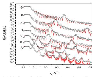
Fig.T.3.2:X-ray reflectivity curves both experimental (open circles) and fitted (solid lines) as a function of wave vector transfer  $'q_z(A^{-1})$  for all samples (A-G)
