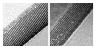
Fig.T.3.6: Cross sectional TEM of sample E (D=2.02nm)and G(D=1.52nm)
