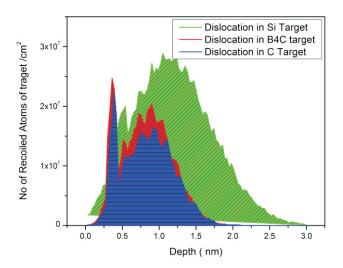
Fig. T.3.3: Damage profile produced due to hitting of 100 eV ions/neutrals on 3 nm layer of Si  $B_4C$  and C layer.
