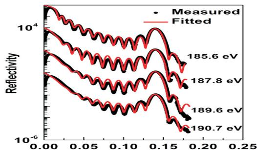
Fig. A.7.1: The measured and simulated RSXR profiles of the C/B<sub>4</sub>C ML, in the vicinity of B K-edge.
