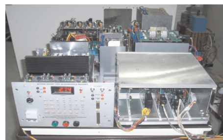
Fig. A.6.4: Active shunt with test magnet.
