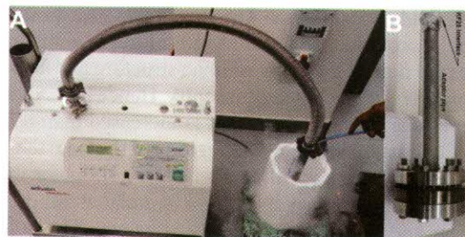
Fig.A.13.3: (A) Helium leak testing of braze assembly at liquid nitrogen temperature (B) Braze assembly
