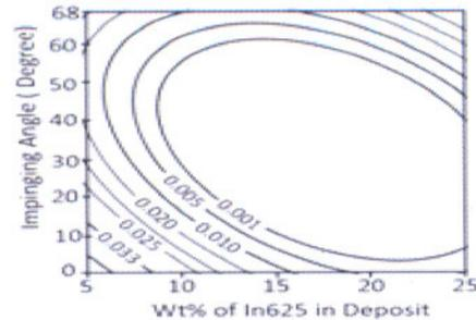
Fig. T.2.4: Contours depicting EWR for various composition and impinging angle at erodent velocity 30 m/s and substrate temperature 150 °C
