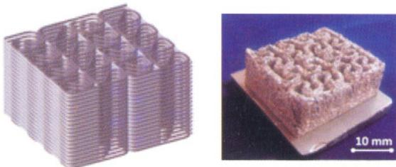
Fig. T.2.9 (a) A typical 3D model (b) Laser rapid manufactured Ti-structure.
