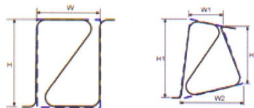
*Fig. T.2.8(a) The unit cell of proposed Z-shaped unit cell based architecture (b) Z-shaped unit cell demonstrating adaptability to various shapes*
