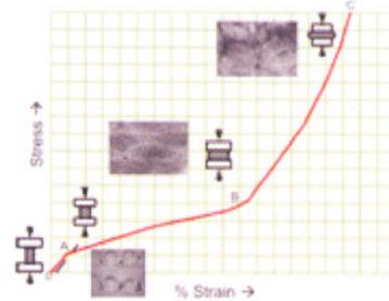
Fig.T.2.10: Typical engineering stress-strain curve obtained during compressive testing of laser rapid manufactured porous Ti-structures
