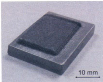
Fig.T.2.2: Typical laser rapid manufactured WC Reinforced Nickel Matrix on 316L SS.
