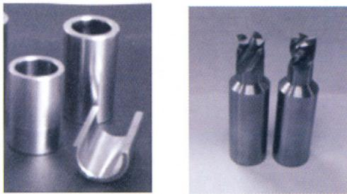
Fig. T.2.5: LRM fabricated (a) Colmonoy-6 bushes (b) WC-Co End-mill
