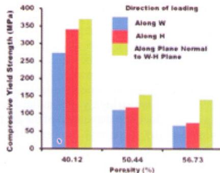
Fig.T.2.11: Compressive yield strength of the laser rapid manufactured Ti-structure at various porosities in different direction of loading.
