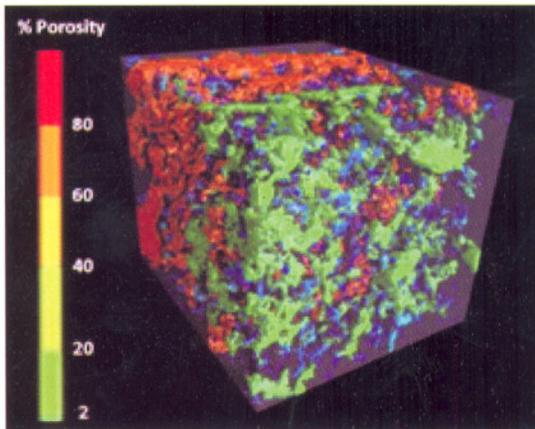
Fig.T.2.12: 3D rendered view of the porous structure exhibiting pore sizes in different color and bulk material in grey color obtained during Micro CT examination.
