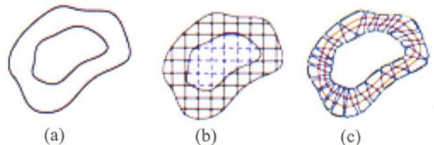
*Fig.T.2.7(a) Typical cross-section of bone, (b) Conventional filling pattern(c) Filling using new Z-shaped unit cell based Architecture*
