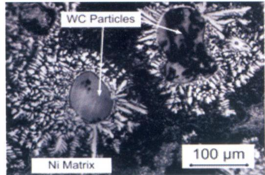
Fig.T.2.3: Micrograph depicting the WC particles in Ni matrix with dendrites.
