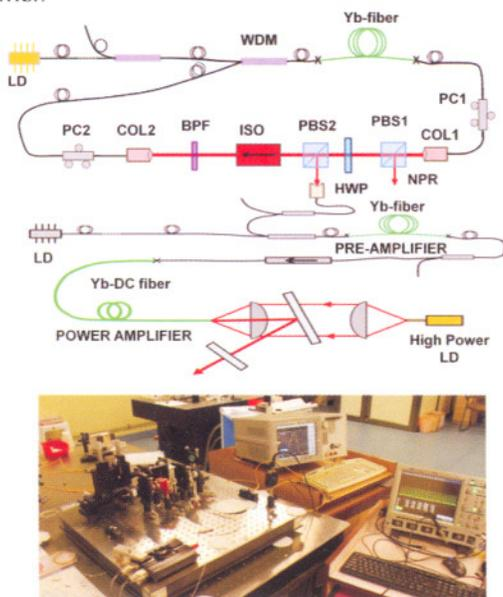
Fig.L.3.1: Schematic (top) and photograph (bottom) of fiber oscillator-amplifier setup.
