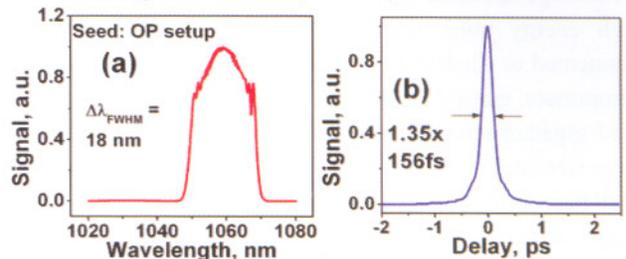
Fig.L.3.2: Recorded (a) spectral profile and (b) autocorrelation trace of the preamplified pulses.
