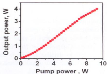
Fig.L.3.3: Variation of amplifier output power with coupled pump power
