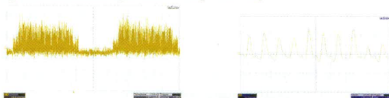
Fig. A.2.3: Typical bunch filling pattern showing 200 filled buckets out of total 291 buckets (left), filling level of individual bucket(right)
