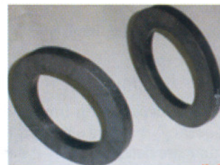
Fig. T.1.10 :Ni-Zn-Co ferrite toroid developed at Ferrite Lab
