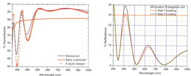
Fig.L.8.3.a) Transmission of bare sapphire, deposited 4 layer structure & calculated transmission spectra, & b) reflectivity spectra of end faces of the coated rod.
