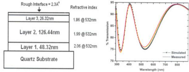
Fig.L.8.2.a) Optical model describing R.I. inhomogeneity, and b) simulated & measured transmission spectra.
