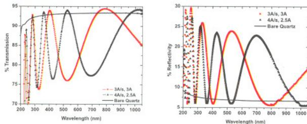
Fig. L.8.1.a) Transmission & b) reflectivity spectra of HfO<sub>2</sub> films grown by ion-assisted e-beam evaporation.
