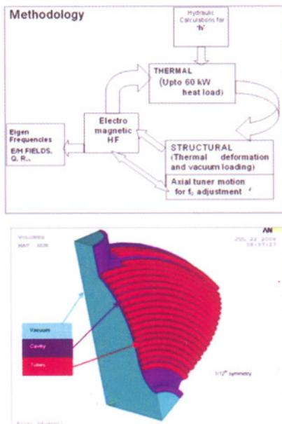
Fig. T.3.3: (a) Coupled sequence cycle for INDUS-2 cavity calculations (top). (b) 1/12th Combined Model of INDUS-2 used for couple analysis (bottom)
