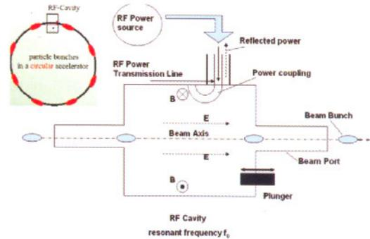
Fig. T.3.1: Particle acceleration in an RF cavity of an accelerator
