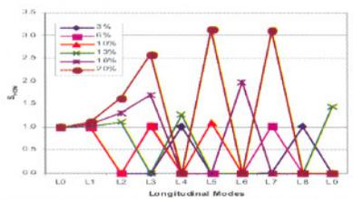
Fig. T.3.10: Effect of increasing iris radius on the characteristic constant (SHOM) for different longitudinal modes.
