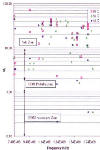
Fig. T.3.6: Matching index for 40°C, 50°C and 60°C of coolant water temperature and 50 mm plunger position for power dissipation of 20 kW.
