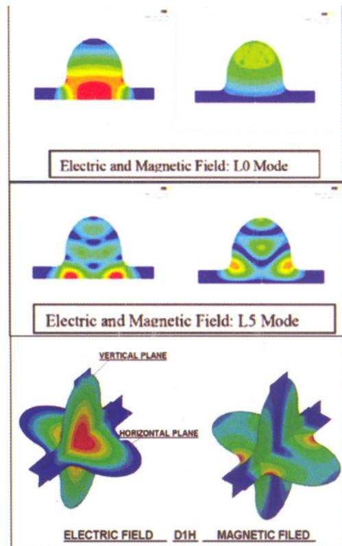
Fig. T.3.2: (a) Resultant Electric (E) and Magnetic field (H) plot of L0 accelerating mode (top), (b) L5 HOM mode (middle) on the RF cavity and (c) D1H HOM mode on the RF cavity. The E field values vary between 0 (blue) and 1 V/m (red) and corresponding H field values vary between 0 and 0.0024 A/m<sup>2</sup>.
