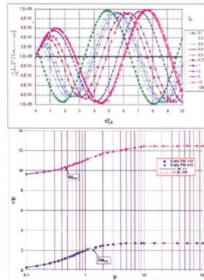
Fig. T.3.7: (a) Plot of the function of derivative of spheroidal radial wave function TM modes are plotted against  $c\xi_0$  by varying  $\xi_0$  from 0.1 to 100, (b) Frequencies in terms of  $c\xi_0$  Vs.  $\xi_0$  for TM modes.
