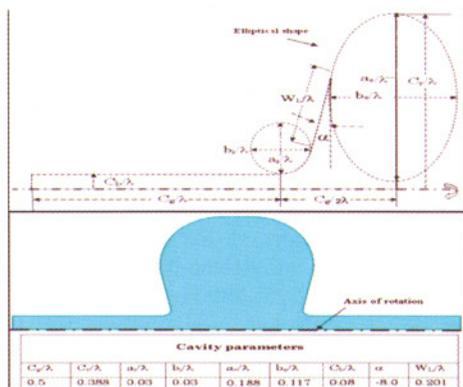
Fig. T.3.9: (a) Parametric dimensions of RF cavity shown by half cylindrically symmetric profile. (b) Optimal profile of the cavity for least number of significant HOMs
