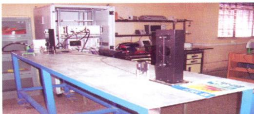
Fig. T.1.17: A multi cell characterization set up for R/Q measurements on prototype 1.3 GHz SCRF cavities.
