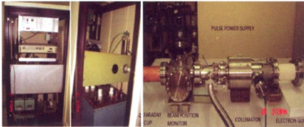
Fig. T.1.19: 55 kV solid state modulator on (left) and high voltage electron gun test set up (right).
