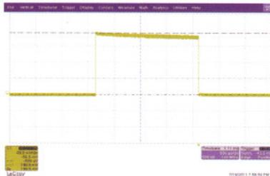
Fig. T.1.25: The 200 W Amplifier system at 1.3 GHz for SCRF cavity tests assembled in a 3U enclosure and output waveform as seen using a microwave diode.
