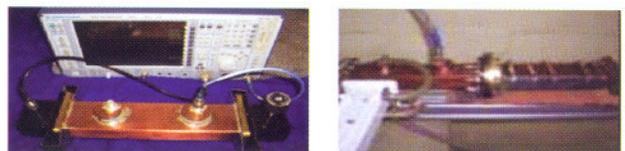
Fig. T.1.13: Left ,loop type dual directional coupler undergoing lower power tests, right SiC load under high power tests on test stand.
