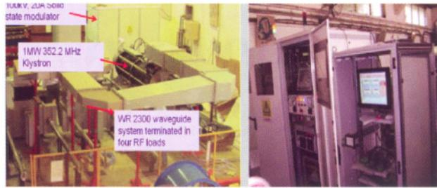
Fig. T.1.21: (Left) 1.3 MW 352.2 MHz Test Stand at RRCAT, (right) the solid state modulator with PC based control system with touch screen GUI.
