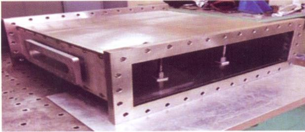
Fig. T.1.15: WR 2300 half height prototype power coupling waveguide developed at RRCAT for LINAC 4 project of CERN.
