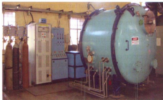
Fig.L.7.1: Renovated 5kW CW CO<sub>2</sub> laser
