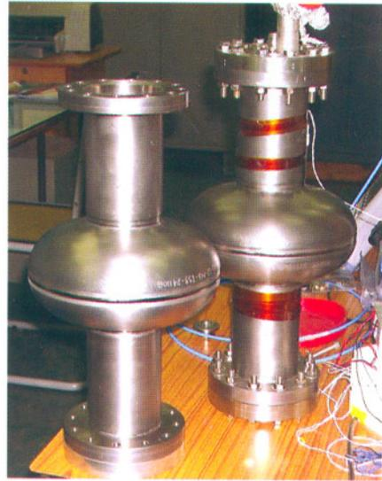
Fig. A.3.1: Prototype cavities undergoing inspection before dispatch to FNAL for processing and performance evaluation
