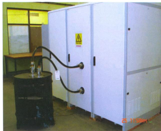
Fig.A.7.2: Evaluation testing of the modulator on a 5kohm, 110kV resistive load
