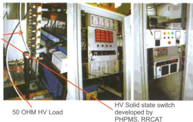
Fig.A.7.1 Modulator Testing on dummy load in primary side with Main & Bouncer IGBT switches
