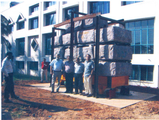
Fig. T.3.1: A test bed at an industry in Bangalore to qualify PMPS jacks
