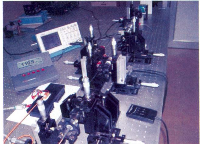
Fig. T.1.4. Photograph of the diode pumped single frequency IR laser at 1064 nm. The power meter display shows ~ 110 mW.
