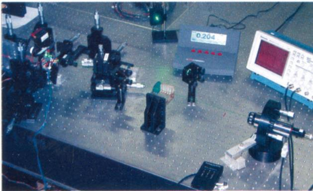
Fig.T.1.6. Photograph of the single frequency green laser at 532 nm operating with ~204 mW output power.
