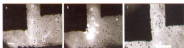
Fig.L.6.2: Sorting of 2 μm diameter polystyrene micro-spheres from a ~50:50 mixture of 1 and 2 μm diameter microspheres. a) 2 μm microspheres are shown by curved arrow and 1 μm microspheres by straight arrow. b) The bright spots are coming from the scattered evanescent field by the microspheres. c) Sorting of 2 μm microspheres into the upward channel by the action of the evanescent field. Increased population of these microspheres can be seen in the encircled region. Scale bar, ~15 μm.
