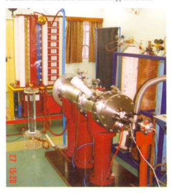
Fig.L.4.1: Photograph of the capillary discharge system.
