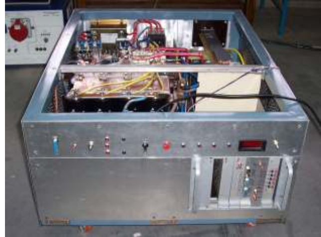
Fig.T.2.7: Photograph of the prototype 30 kVA inverter.
