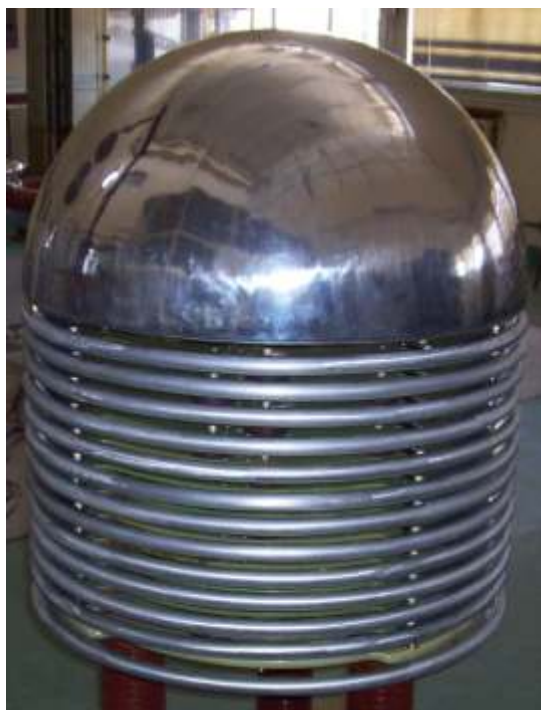
Fig.T.2.9: 300 kV multiplier stack assembly for SLEA
