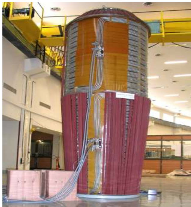
Fig.T.2.5. Primary windings of the HPIA being tested at RRCAT
