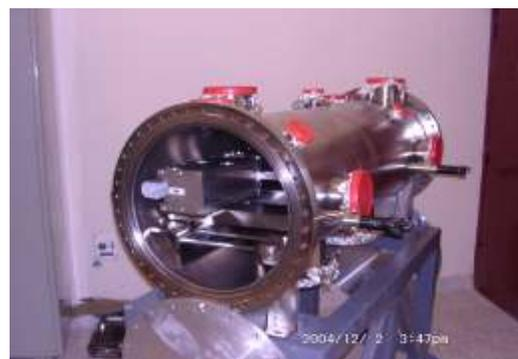
Fig T.2.4 Injection septum chamber with septum magnets
