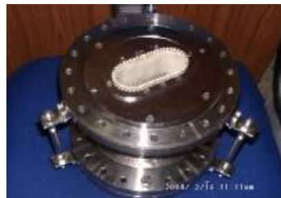
**Fig T.2.7** RF-shielded bellow assembly
