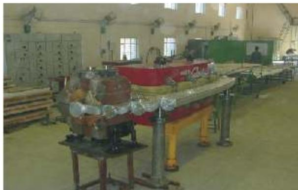
Fig T.2.2 Assembled BM chamber
